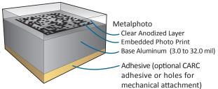
materials. An optional CARC adhesive is also available. The label has excellent resistance to chemicals, abrasion, solvents; and will withstand exterior exposure in the harshest environments, including extreme cold, heat and UV. When treated with our image intensification process, Metalphoto's expected exterior life exceeds 20 years.
